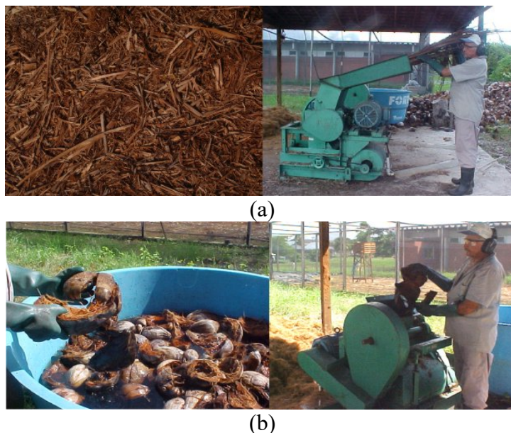
Figure 33. A) Crusher of dry coconut shell, B) immersion of shell in water to be crushed
