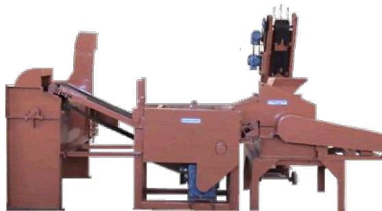
Figure 32. Equipment for processing green coconut shell
