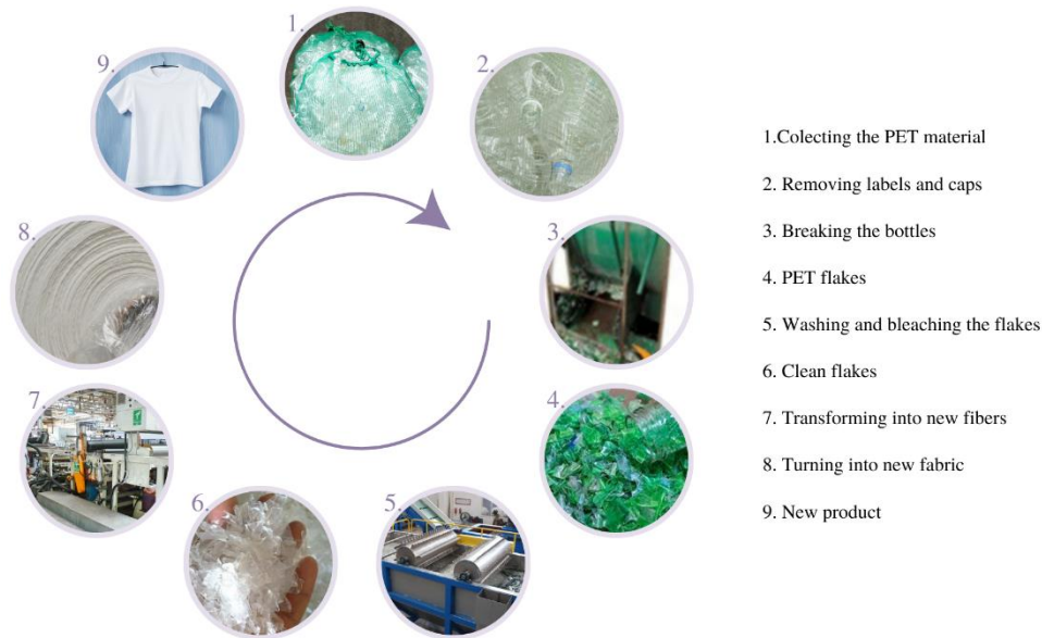
Figure 26 – Production Cycle of a PET textile
