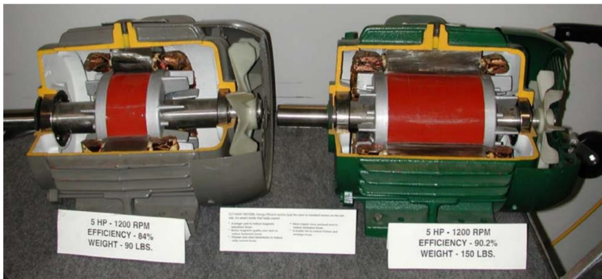
Figure 22. The difference in the material quantity between Standard SCIM and High-Efficiency SCIM. Source: [98].
