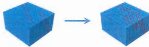
Figure 37 - Example of process of damage evolution through increase in crack density in the microscale model for a [\pm 60^\circ_4]_s laminate
