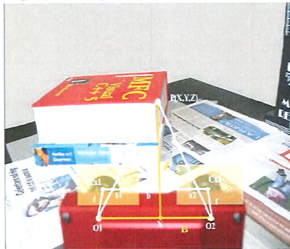
Figure 17 – Disparity and depth in stereo vision
