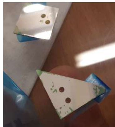
Figure IV-9 - Metalenses with aluminium apertures fabricated with lift-off technique.
