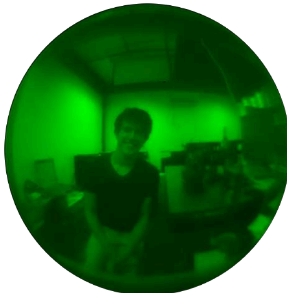
Figure IV-19 – Photo taken with WFOV metalens camera under incoherent illumination (ambient light). To minimize the chromatic aberration, a green filter was used.
