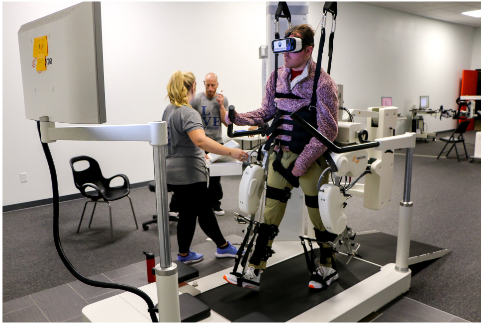
Figure 4 – Patient wearing the Lokomat robotic exoskeleton and performing treadmill walking with a HMD, a common setup to achieve infinite straight walking in VR.
