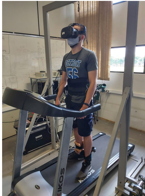
Figure 41 – Subject wearing the HMD and the lower limbs exoskeleton on the treadmill during the tests.
