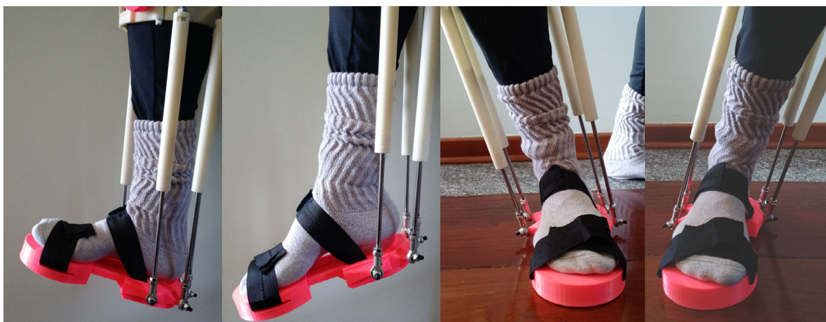
Figure 28 – Test subject performing the four anatomical ankle motions. From left to right: dorsiflexion, plantarflexion, eversion and inversion.
