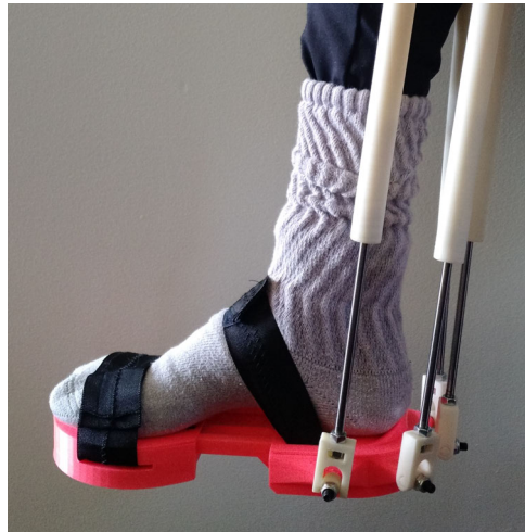
Figure 30 – Complete prototype with spherical rod ends replaced by custom universal joints.
