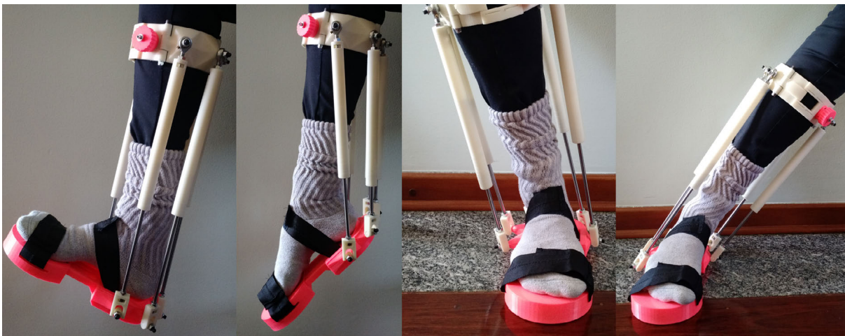
Figure 31 – Four anatomical motions performed with universal joints installed. From left to right: dorsiflexion, plantarflexion, eversion and inversion.
