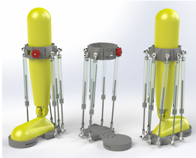
Figure 25 – Final CAD design of the parallel ankle joint prototype.
