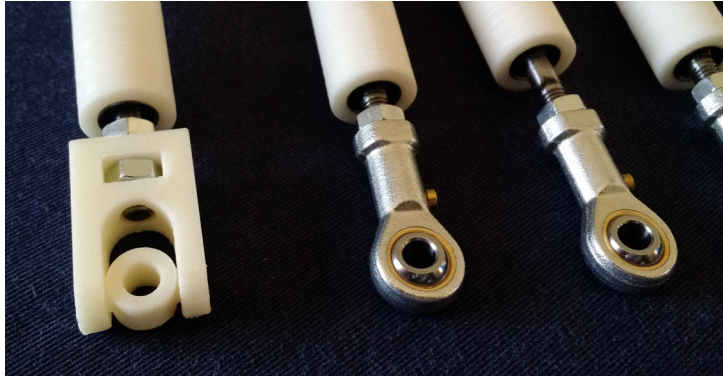
Figure 29 – Custom universal joint (left) side by side with the commercial spherical rod ends (right), connected to the lower extremity of the linear actuators.
