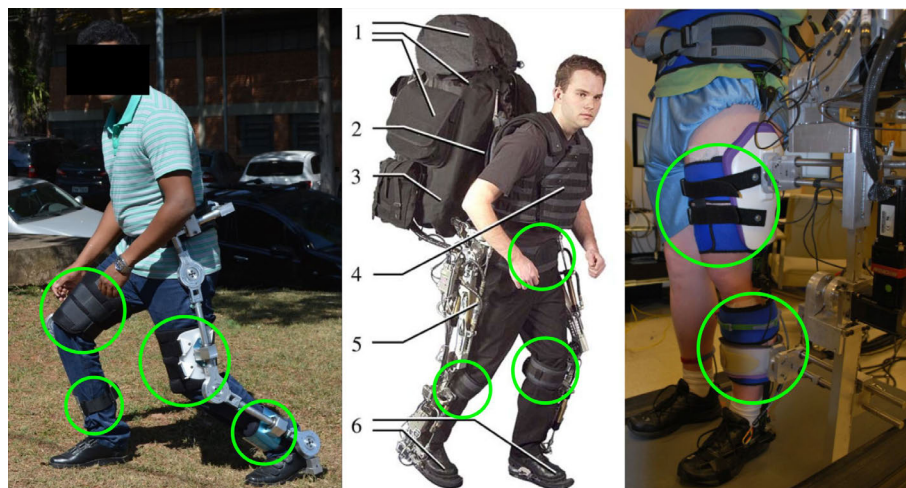
Figure 5 – From left to right: EXO-TAO, BLEEX and ALEX II. Notice the recurrent usage of straps (marked in green) to connect the exoskeleton to the human user.
