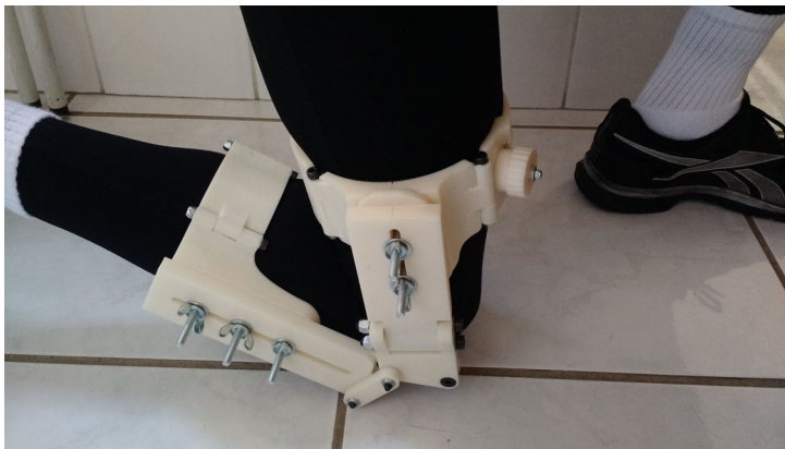
Figure 52 – Genuflexion while wearing the external knee joint. The proposed geometry, with the joint not covering the patella region, does not interfere on such posture.
