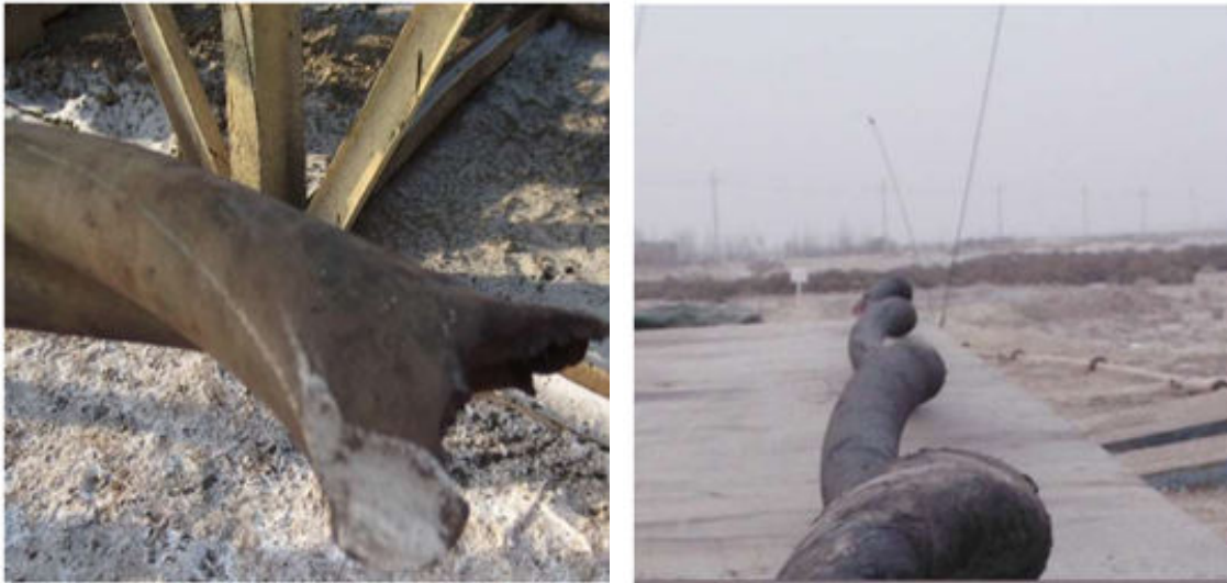
Figure 9 – Tubing damage caused by perforating gun shock.
