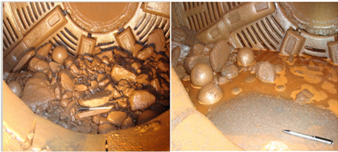
Figure 9. Typical mill loads as observed in pilot scale tests: open circuit (left) and closed-circuit (right) SAG operation (modified from Rodrigues, 2014)
