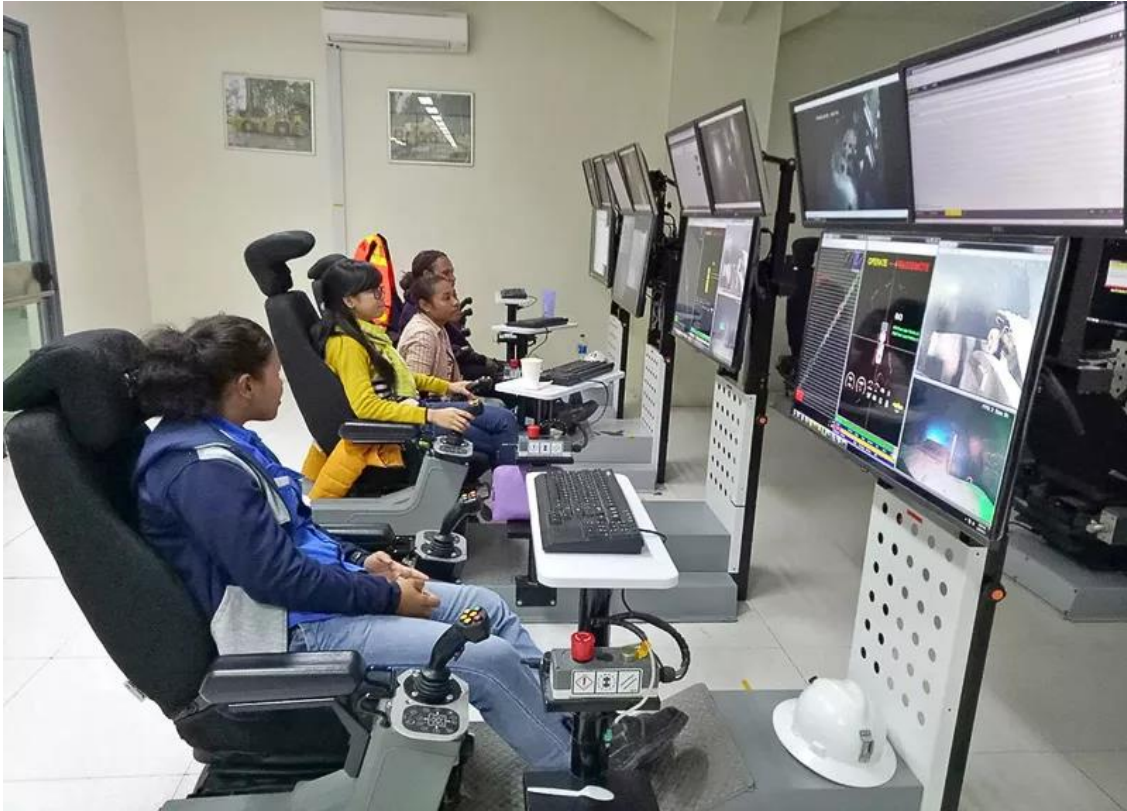
Figure 3 Remote operations control room ( www.immersivetechologies.com/products/Remote-Operation-Technologies.htm ).
