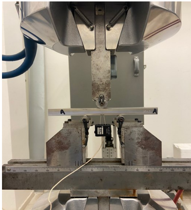
Figure 28: SE(B) specimen of 316L stainless material in the MTS machine during the fatigue crack propagation test.
