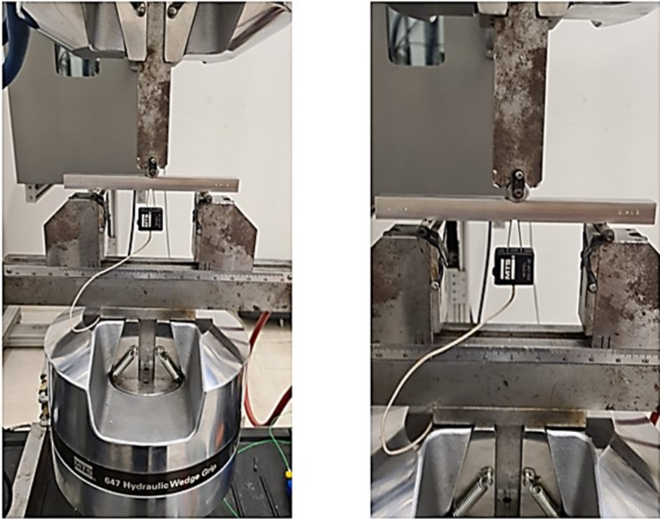
Figure 48: SE(B) specimen machined from AISI 316L stainless steel mounted in MTS test machine during fatigue crack propagation testing for S/W = 8 .
