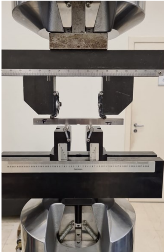
Figure 50: SE(B) specimen machined from AISI 316L stainless steel mounted in MTS test machine during four-point bend compressive precracking.
