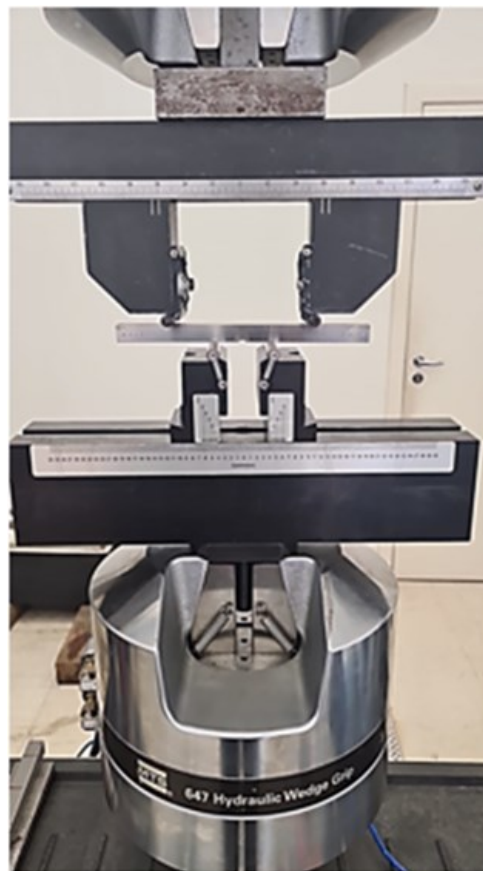
Figure 52: SE(B) specimen machined girth weld mounted in MTS test machine during four-point bend compressive precracking.
