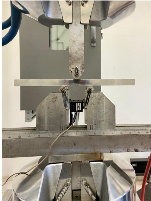
Figure 27: SE(B) Specimen of AISI 316L material in the MTS machine during the fatigue crack propagation test with S/W=4 .
