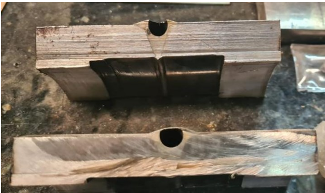
Figure 45: Specific shape where were machined the specimens for tensile tests.
