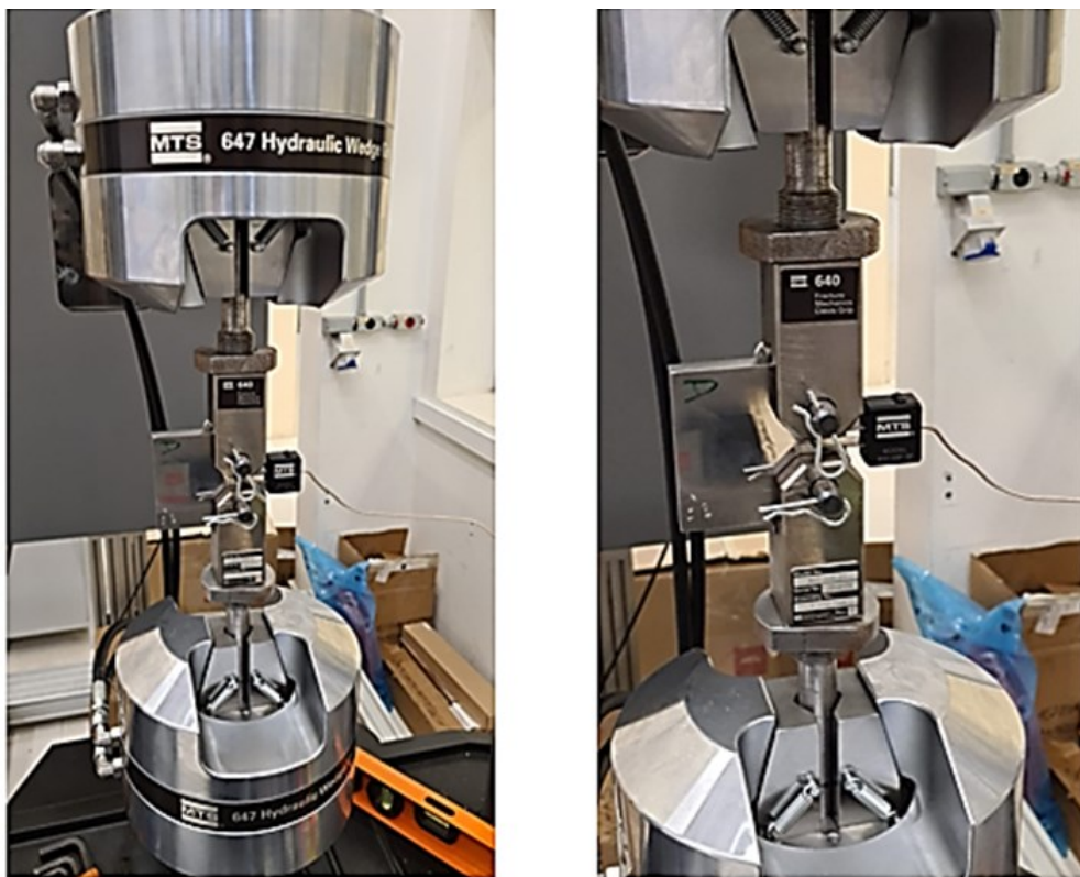
Figure 46: C(T) specimens machined from AISI 316L stainless steel mounted in MTS test machine during fatigue crack propagation testing.
