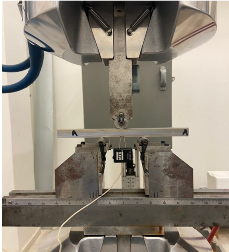
Figure 49: SE(B) specimen of 316L stainless material in the MTS machine during the fatigue crack propagation test.
