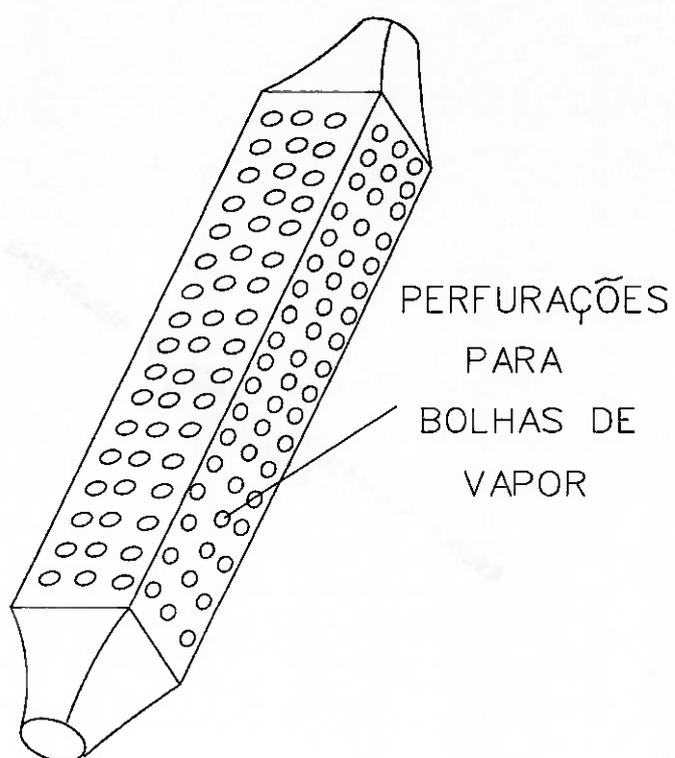
FIGURA 3.2.1.2. ELEMENTO COMBUSTÍVEL DE REATOR BWR
