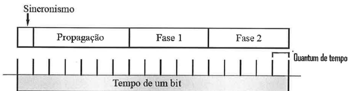
**Figura 3.5 – Segmentos do *bit* transmitido**
