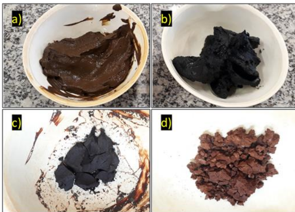
Figure 34 - Samples for OM tests by ignition at 440 °C: a) Cubatão-WTS before ignition; b) Taiaçupeba-WTS before ignition; c) Cubatão-WTS after ignition; d) Taiaçupeba-WTS after ignition.
