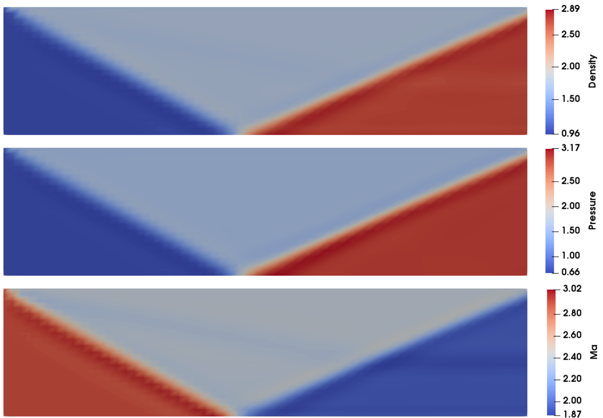
Figure 5.3 – Solution obtained for Density, Pressure and Mach number in the shock reflection problem
