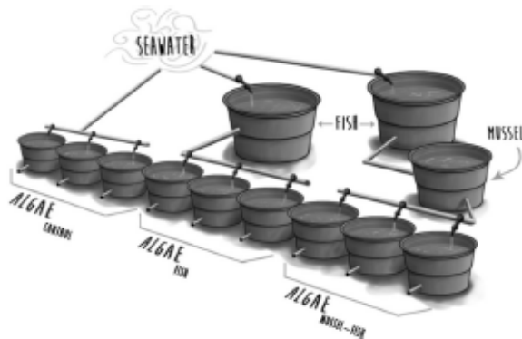
Fig. 1 General scheme of the integrated multi-trophic culture system, showing the treatments: control Algae (A), Algae + Fish (AF), and Algae + Mussels + Fish (AMF)
