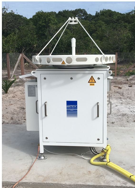
Figure 4: Photo from Mira 35-C, the cloud radar located at the Campina site. Adapted from https://www.attoproject.org/cloud-radar-measuring-from-a-hole-in-the-forest/ .
