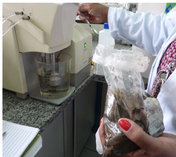
Figura 12 - Granulometria à laser – Malveer Mastergizer
