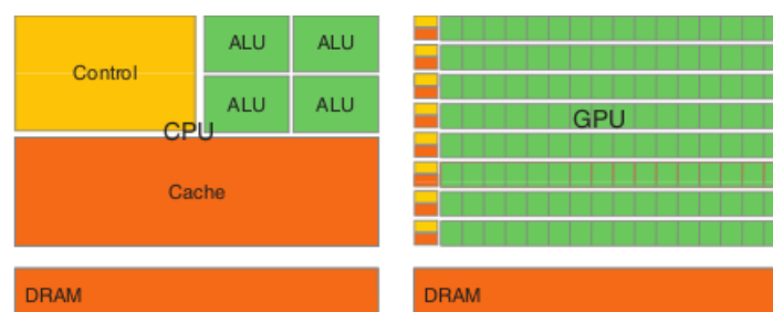
Figure 2.8: A comparison of the schematic architectures of CPUs and GPUs. Taken from Kirk and Hwu [2013]
