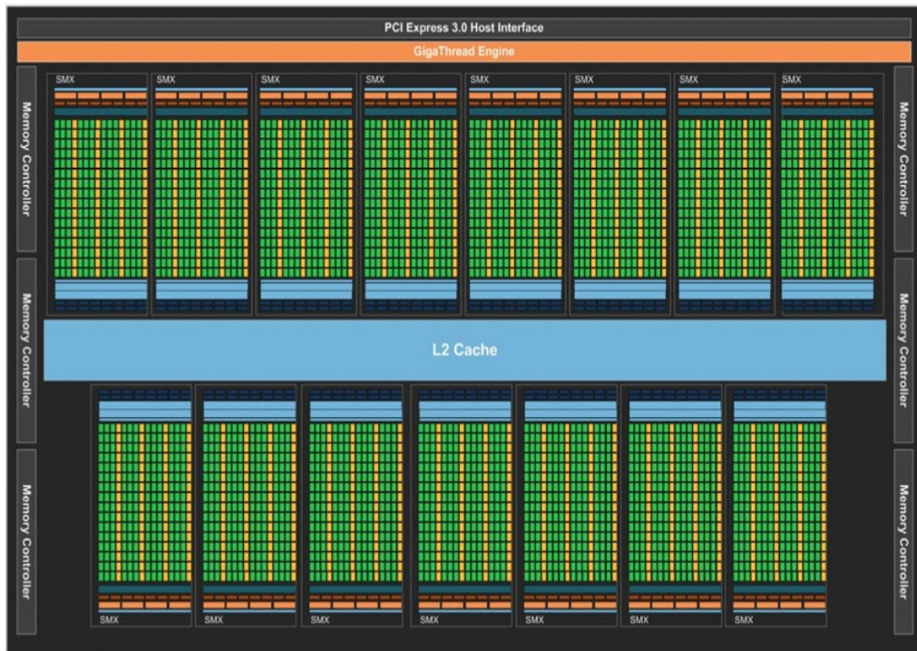
Figure 2.10: Block diagram of the GK110 chip architecture. Taken from NVIDIA [2012].
