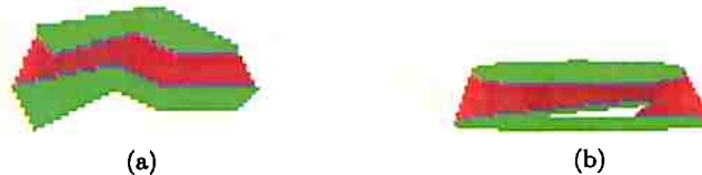
Fig. 2. (a) Region between two objects, calculated by the visibility approach; (b) Analogous to (a), but showing that the concavity of one of the objects is properly excluded from the between region by the visibility method.
