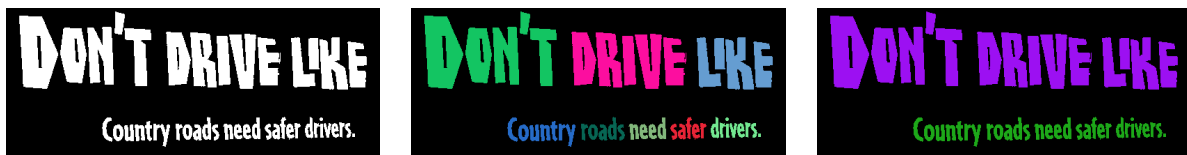
Figure 5.3: Extraction of letters, words and lines of text using different thresholds for the variance of the distance of merged nodes, based on the component-hypertree from Fig. 5.2. For example, by selecting nodes with variance less than 0.3, words can be extracted (middle column, where elements with the same color belong to the same node) and, if no threshold is given, then entire lines of text can be obtained (right).
