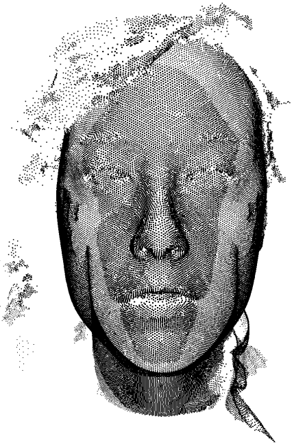
(c) Point cloud extracted from original mesh.
