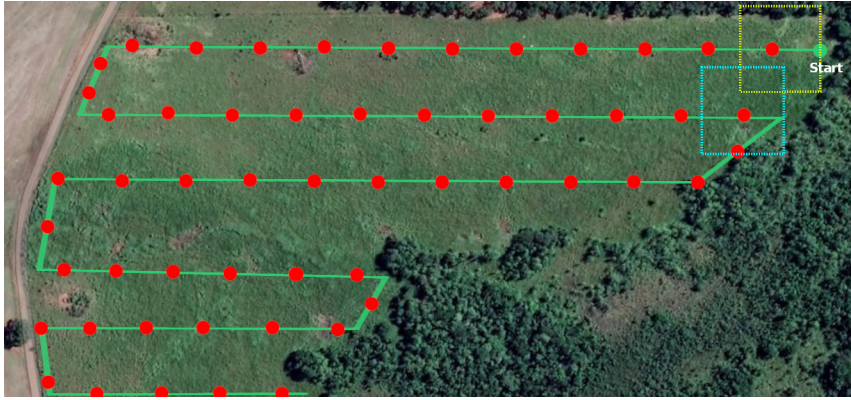
Figure 27 – Drone’s flight plan illustrating the path (green line) and photo capture locations (red dots) for a pasture area. The yellow and blue dotted boxes represent adjacent photos taken with a significant time lapse.
