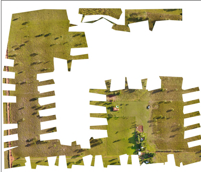
Figure 26 – Example of unsuccessful orthophoto generation due to low overlap between images.
