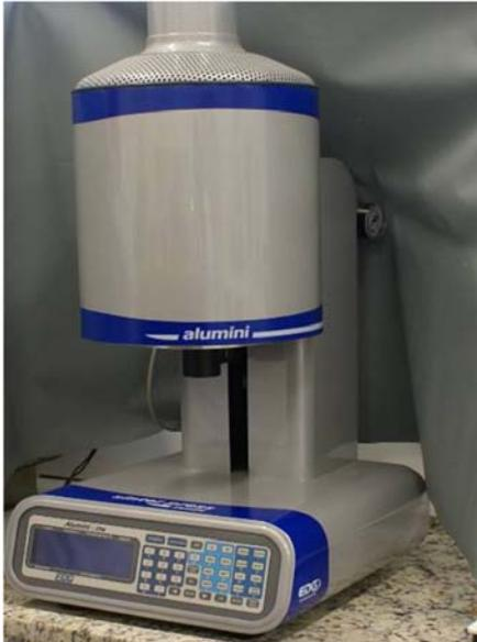
**Figura 14** - Forno Alumini-Sinter Press
