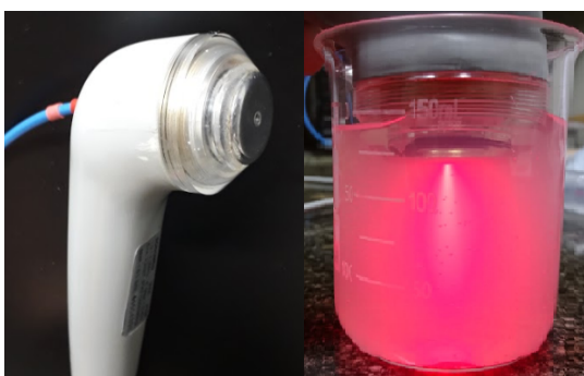
Figure 27 – The sono-photodynamic probe is composed by an ultrasound transducer with the implementation of a UV-Visible optical fiber positioned in the middle.
