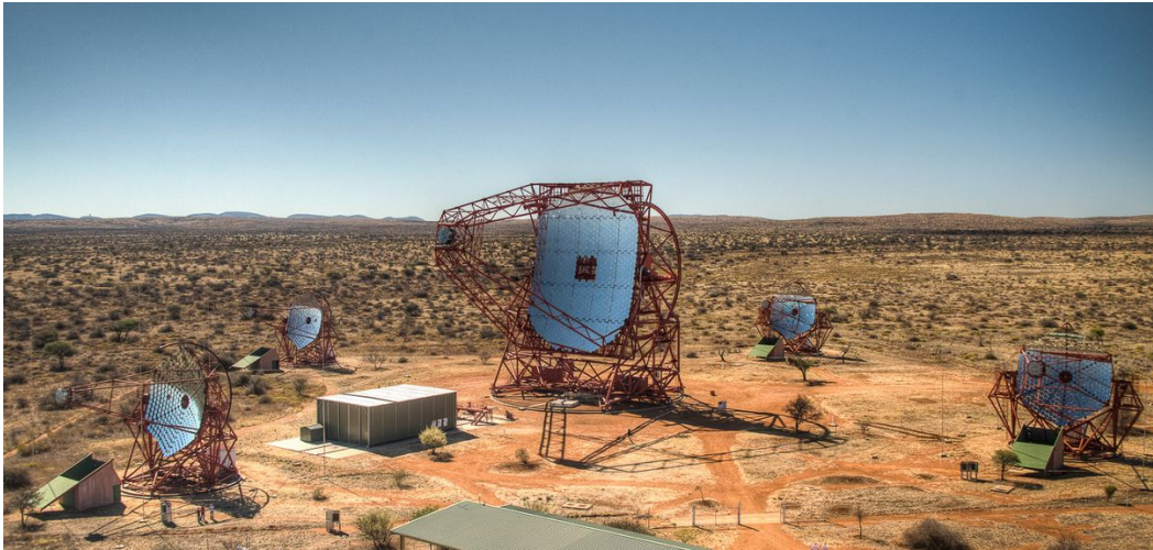
(a) Picture of the 28 and the four 12-meter telescopes of HESS, in the Namibian desert. Image credit: HESS Collaboration. Available at: https://www.mpi-hd.mpg.de/HESS/pages/home/Webgalleries/HESS2_telescope/index.html . Accessible at: Jan 16.
