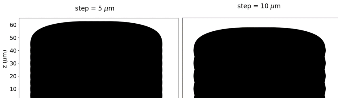
Figure 3.2 - Representation of a wall of a cylindrical structure in the z-direction, considering two different z-step parameter values. It is possible to note that a non-ideal parameter leads to a wall with high surface roughness, which can scatter light and introduce optical losses.
