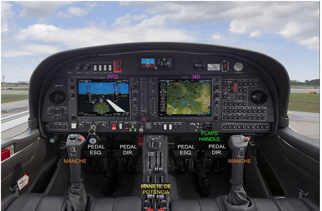
Figura 2. Cockpit da aeronave Diamond DA42. Disponível em: https://www.diamondaircraft.com/en/private-pilots/aircraft/da42/overview/ .
