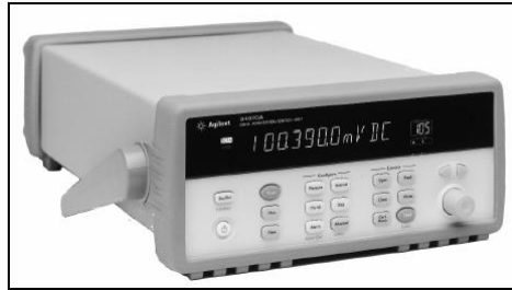
Foto: HP34970A Data Acquisition / Switch Unit User's Manual Figura 3.10. Datalogger HP34970
